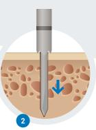
Tunnel creation with the drill or the tap to the laser marking
